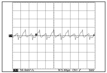
Figure 16: Output voltage ripple at nominal input voltage and rated load current (50 mV/div). Load capacitance: 1µF ceramic capacitor and 15µF tantalum capacitor. Bandwidth: 500 MHz. See Figure 13.
