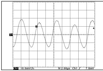
Figure 14: Input Terminal Ripple Current, i<sub>c</sub>, at full rated output current and nominal input voltage with 10µH source impedance and 47μF electrolytic capacitor (100 mA/div). See Figure 13.
