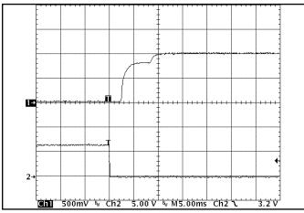
Figure 9: Turn-on transient at full rated load (resistive load) (5 ms/div) Input voltage pre-applied. Ch 1: Vout (500mV/div). Ch 2: ON/OFF input (5V/div)
