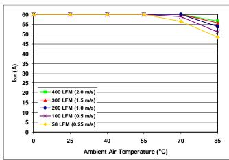
Figure 5: Maximum output power derating curves vs. ambient air temperature for airflow rates of 50 LFM through 400 LFM with air flowing across the converter from pin 3 to pin 1 (nominal input voltage).
