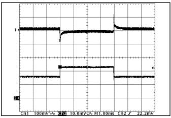
Figure 12: Output voltage response to step-change in load current (50%-75%-50% of Iout(max):  $dI/dt = 5A/\mu s$ ). Load cap:  $470\mu F$ , 30 m $\Omega$  ESR tantalum cap and 1µF ceramic cap. Ch 1: Vout (100mV/div), Ch 2: Iout (20A/div).
