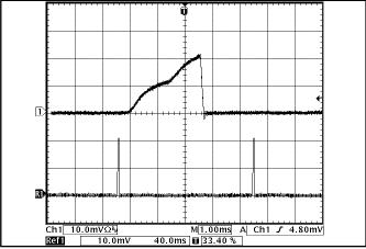
Figure 18: Load current (50A/div) as a function of time when the converter attempts to turn on into a 1 m $\Omega$  short circuit. Top trace (1.0ms/div) is an expansion of the on-time portion of the bottom trace.
