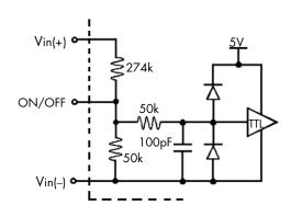
Figure B: Internal ON/OFF pin circuitry
