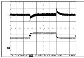
Figure 11: Output voltage response to step-change in load current (50%-75%-50% of Iout(max);  $dI/dt = 0.1A/\mu s$ ). Load cap:  $10\mu F$ ,  $100 \, m\Omega$  ESR tantalum cap and 1µF ceramic cap. Ch 1: Vout (50mV/div), Ch 2: Iout (20A/div).
