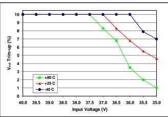
Figure 23: Achieveable trim-up percentage vs. input voltage. at +85°C, +25°C and -40°C (all at full load). Full trim-up percentage is achieved at loads of 50% or less across full temperature range.
